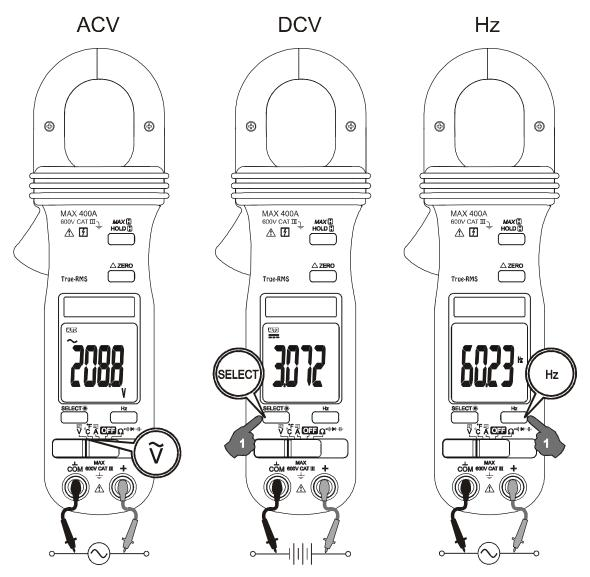
Set slide-switch to Voltage function position. Inputs are made through the test leads terminals. For Models 063 & 065, slide-switch on defaults at AC voltage. Press **SELECT** button momentarily to select DC voltage. For Models 061& 062, separate ACV & DCV slide-switch positions are being used.
